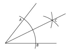
This uses the principle of **Balance**. An arc is drawn, cutting the two lines at *A* and *B*. With *A* and *B* as centres, two equal arcs are drawn intersecting at *C*. The angle bisector is the locus of points equidistant from the two lines.
