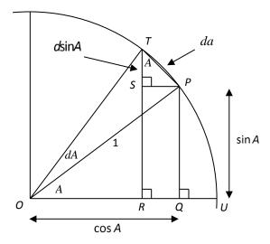
In the unit circle above  $\cos A$  and  $\sin A$  are as shown and since  $\angle OPS = A$ , then  $\angle STP \approx A$  as  $\angle OPT$  is approximately a right angle and approaches a right angle as dA approaches zero.
